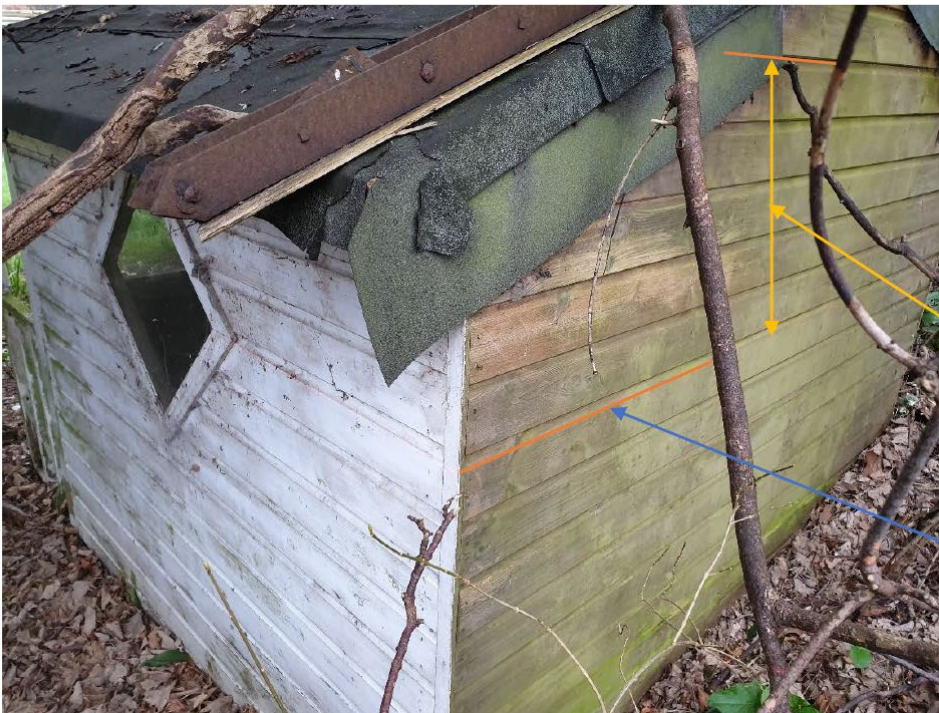
This picture has the laser level line from the front door threshold of 29 Westcote Road projected onto the rear of the summer house showing that it is ~0.5m below the 18/16 Parkside Road fence line.
